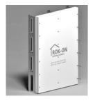
ROK-ON™ Structural Insulated Sheathing (SIS) consists of one layer of ROK-ON™ FRCC 12mm structural sheathing and a layer of 6mm FRCC bonded to an insulating EPS or phenolic foam core. The sheathing panel is up to R-21, exceeding the requirements for continuous insulation in the building code across North America.
